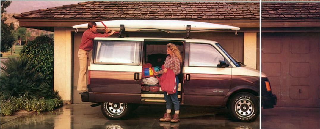
Long loads on the roof don't interfere with back-door operation, thanks to Astro's swing-out rear doors. There's no lift-gate to stretch for and no tailgate to reach over. The rear step bumper also facilitates roof-top loading. Shown at right, Astro with optional CS trim in optional Special Two-Tone Tan and Burnt Red Metallic. Tires supplied by various manufacturers.
