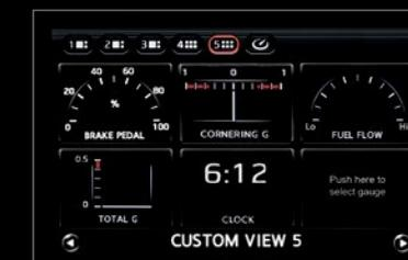
**Factory preset screen.** For proof of the GT-R's dedication to performance, look no further than the factory preset screen – a dedicated stopwatch activated from the steering wheel. You can even store your track times on a flash drive using the USB port in the center console.<sup>1,2</sup>
