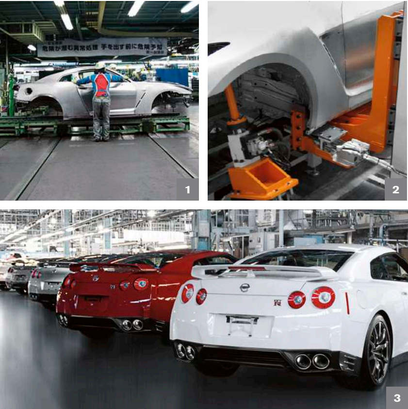
1_ Every GT-R receives a high degree of hand-assembly and finishing. 2_ Vibration testing, laser measurements, and comprehensive inspections by experienced specialists are performed to ensure long-term functionality and to maintain the highest levels of accuracy and precision during assembly. 3_ After a hand-finishing of the body panels and careful polishing, the GT-R is ready.
