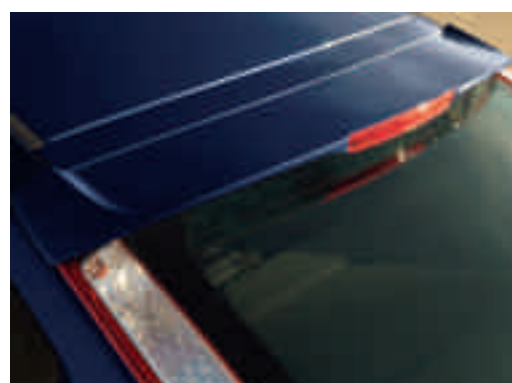
Body colour rear spoiler Aerodynamically-styled for a competitive edge.
