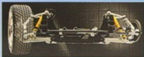
RACING-INSPIRED FRONT SUSPENSION The Corvette front suspension features high-strength forged-aluminum componentry and quick-ratio power rack-and-pinion steering.
