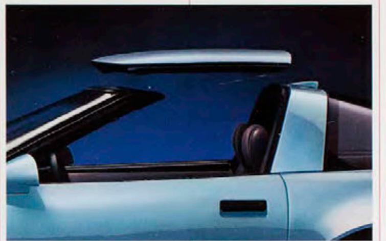
Corvette Coupe features a standard removable roof panel (one-piece with no center T-bar).
