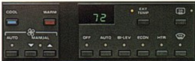
New electronic air conditioning features fingertip push-button control.
