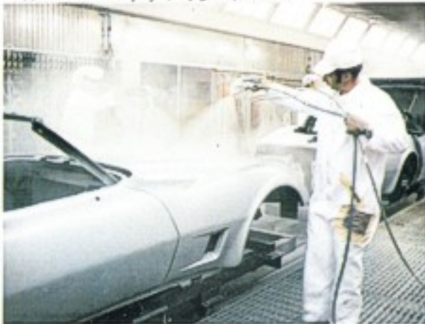
The first of six coats of color is applied to the body by spray gun specialists.
