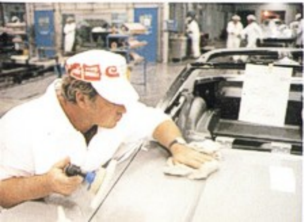
After a final clear coat, the finish is hand-polished and imperfections noted and removed.
