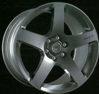
FIVE SPOKE Durabright, forged aluminum Front: 18" x 10" / Rear: 19" x 13"
