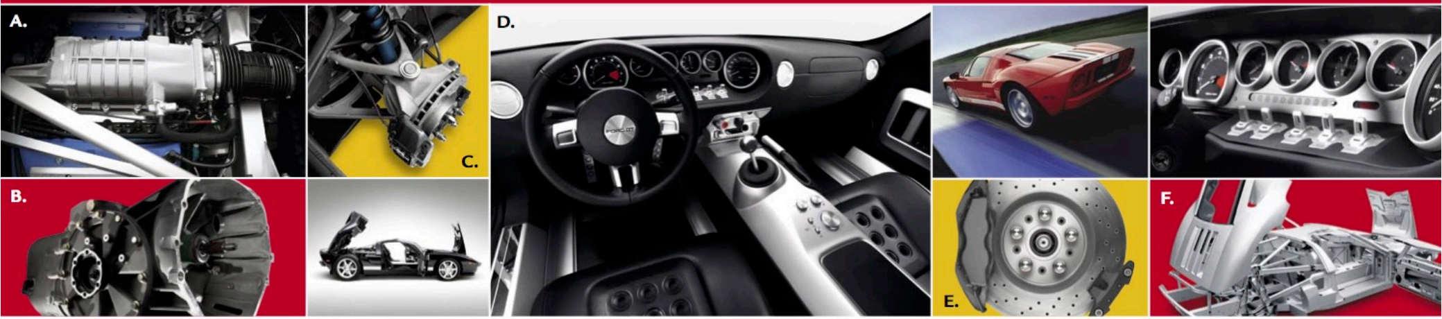
A. A mid-mounted, all-aluminum 5.4L DOHC supercharged V-8 engine that produces 550 horsepower. B. A six-speed Ricardo transaxle with twin-disc clutch and limited-slip differential. C. A race-inspired, double-wishbone front and rear suspension that contributes to Ford GT's exceptional handling and ride quality. D. A computer-modeled interior design that recalls the original Ford GT40. E. Massive 14-inch front and 13-inch rear disc brakes that feature four-piston aluminum calipers and cross-drilled and vented rotors to provide maximum braking performance. F. An aluminum space frame combined with Super Plastic Formed (SPF) aluminum body panels and extensive use of carbon fiber for strength and lighter weight.
