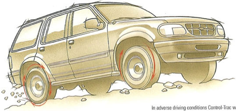
In adverse driving conditions Control-Trac will distribute torque to the wheels, adjusting for loss of traction.
