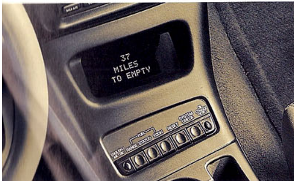
to premium console, equipped with message center, monitors 30 vehicle activities, including minders for your next oil change.
