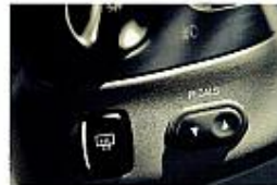
Class exclusive: Optional power adjustable pedals can be easily adjusted by the switch conveniently located on the instrument panel.
