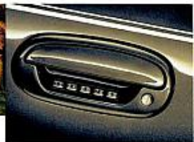
Keyless entry pad system allows you the convenience of unlocking your doors without the use of a key or key fob.
