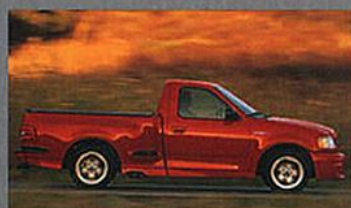
1999 SVT F-150 LIGHTNING 360 horsepower supercharged 5.4-liter Triton™ V8 Four-wheel disc brakes introduced 5,000-pound tow rating Production: 4,000 units (estimate)
