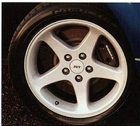
The Cobra forged 17 x 8 in. aluminum-alloy wheels are shod with 245/45-17 BFGoodrich™ Comp T/A ZR tires.
