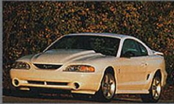
1995 SVT MUSTANG COBRA R 300 horsepower 5.8-liter ohv V8 Tremec five-speed manual transmission Lightweight street-legal racing model Production: 250 units
