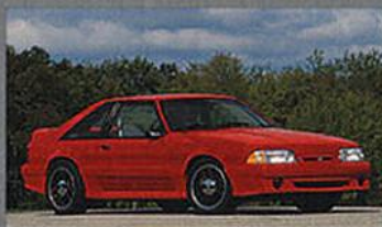
1993 SVT MUSTANG COBRA R 235 horsepower 5.0-liter ohv V8 T5 five-speed manual transmission Lightweight street-legal racing model Production: 107 units
