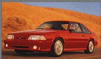
1993 SVT MUSTANG COBRA 235 horsepower 5.0-liter ohv V8 T5 five-speed manual transmission Four-wheel disc brakes Production: 4,993 units
