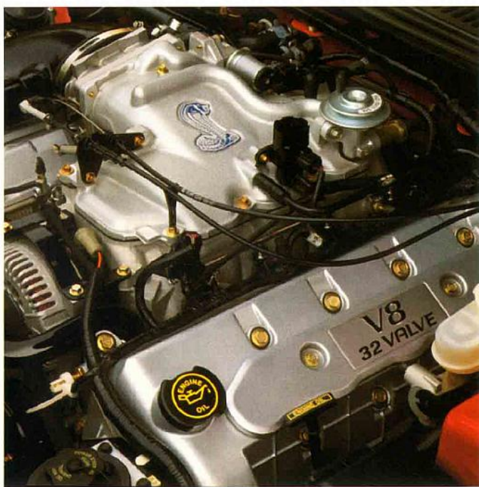
Top: Two-person teams assemble the SVT Cobra V8s on a dedicated Niche Line. When the engine is completed, the two builders scribe their names into an aluminum badge that is then affixed to the right cam cover.
