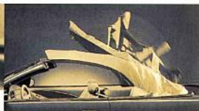
The hydraulic convertible top is designed to allow approximately 30% faster raising and lowering times than before.
