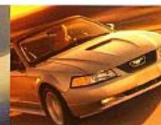
Mustang GT convertible in Chrome Yellow Clearcoat Metallic. The updated modular 4.6-liter single-overhead-cam V8 makes 260 horsepower with 302 lbs.-ft. of torque.
