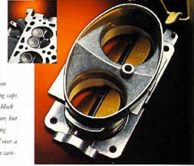
Right: The specially designed Cobra throttle body has twin 57mm bores. Inset, right: The Cobra combustion chamber
