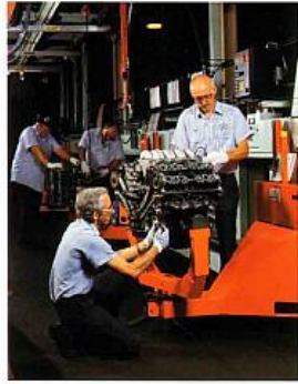
Above: The SVT Cobra engine is assembled at the Ford Romeo Engine Plant on a dedicated Niche Line staffed by 12 two-person teams. When a team completes an engine, both assemblers scribe their names into an aluminum badge that is then affixed to the right cam cover. Right: Cobra alloy pistons feature a 9.85:1 compression ratio. The connecting rods are sinter-forgings, with fracture-split big ends.
