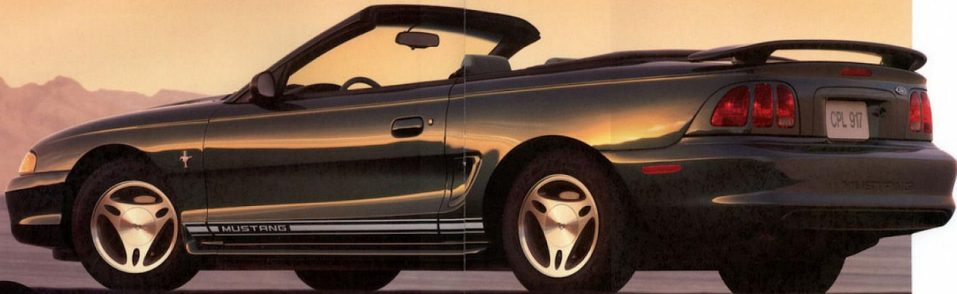
LEFT: Mustang is powered by a 150-hp 3.8-liter SEFI V6. All Mustangs come with a standard passive anti-theft system.
