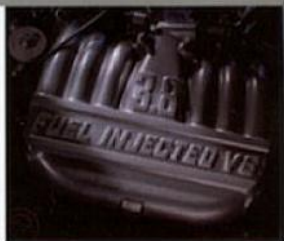
LEFT: Mustang is powered by a 150-hp 3.8-liter SEFI V6. All Mustangs come with a standard passive anti-theft system.
