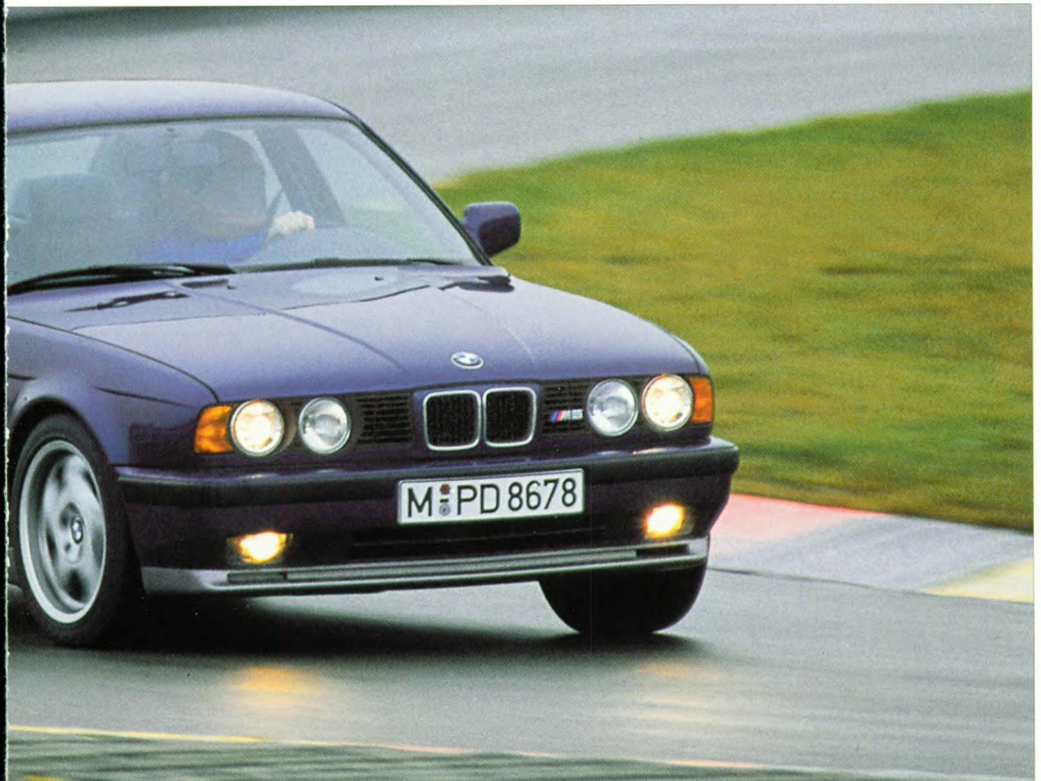
with extremely agile handling and equally dynamic cornering (switch position P = automatic suspension tuning, S = sports tuning). The final touch is provided by the extra-strong anti-roll bar at the rear, 9 J x 17 wheels with 225/40 ZR 17 rear tyres, and special Servotronic power steering tuned for performance motoring.
