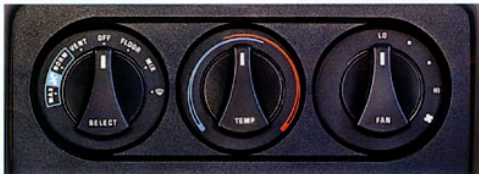
Air conditioning with rotary controls.
