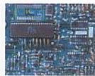
Ford's new EEC-IV computer provides precise and instantaneous control over vital engine functions.
