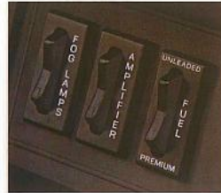
Fuel recalibration from premium to regular unleaded is accomplished by a flick of a switch on the console.
