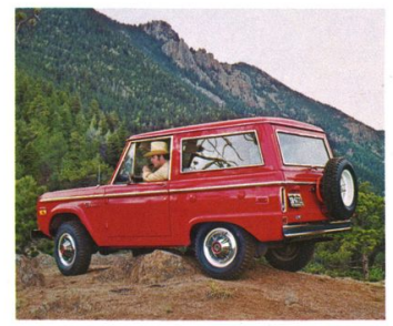
Excellent ground clearance. Bronco combines optimum ground clearance amidships with a big ramp breakover angle to allow crossing over high projections. Bronco's excellent angles of approach and departure provide greater freedom from hangups when approaching or leaving steep inclines and ditches.
