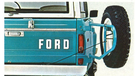
Swing-Away Spare Tire Carrier puts spare out of the way for more cargo or luggage area, easier access.
