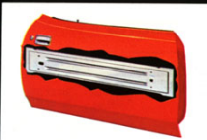
Steel Guard Rail —standard on all 1971 Mustangs. Steel box-section door beams help absorb side impact forces.
