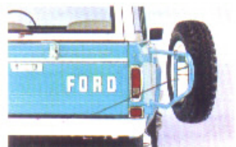
Swing-Away Spare Tire Carrier gets the tire out of the way for more cargo area, easier access.
