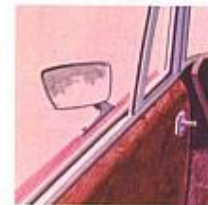
Remote-Control Outside Rearview Mirror. Provides clear view of approaching traffic and makes it easy to set the mirror at the most desirable angle. Without lowering the window, you can aim the mirror by moving the inside fingertip control.
