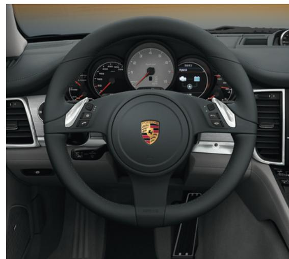
Three-spoke sports steering wheel with gearshift switches
