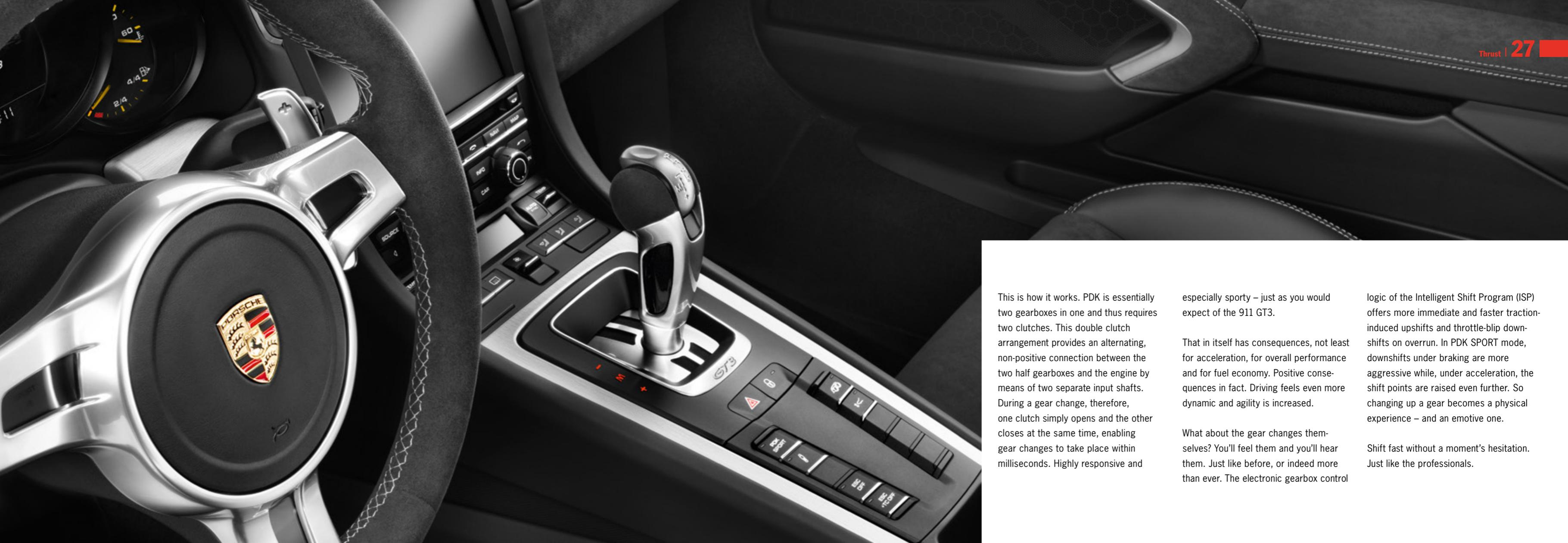
This is how it works. PDK is essentially two gearboxes in one and thus requires two clutches. This double clutch arrangement provides an alternating, non-positive connection between the two half gearboxes and the engine by means of two separate input shafts. During a gear change, therefore, one clutch simply opens and the other closes at the same time, enabling gear changes to take place within milliseconds. Highly responsive and
