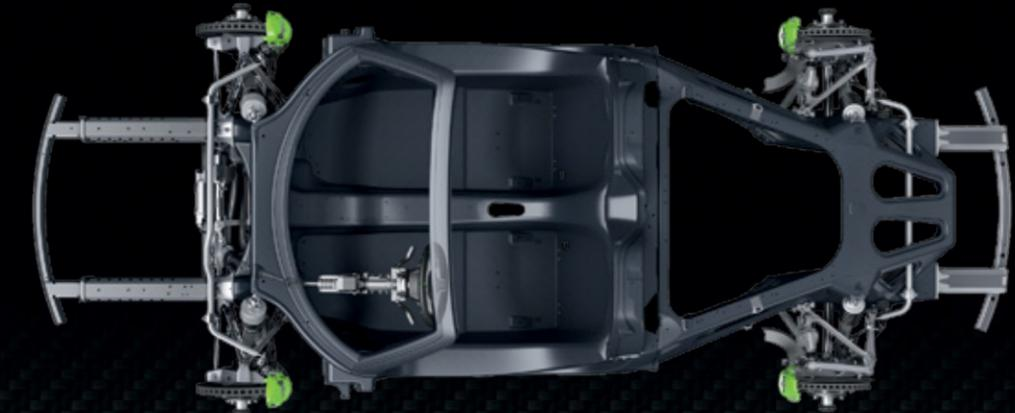
Monocoque and unit carrier
